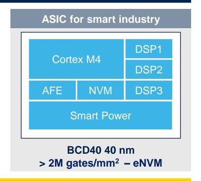
Digitally-managed power provides configuration, monitoring and supervisory functions to meet advanced system needs
